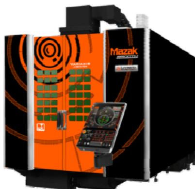
**VARIAXIS j-600 AM equipped with Wire Arc metal deposition**
