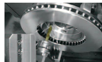
Brake disk machining by IVS
