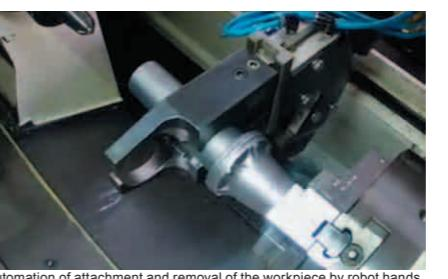
Automation of attachment and removal of the workpiece by robot hands
