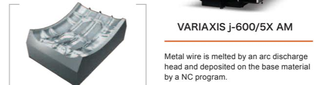
Metal wire is melted by an arc discharge head and deposited on the base material by a NC program.
