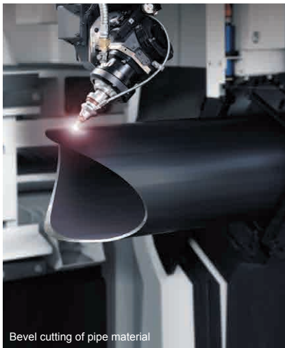
Bevel cutting of pipe material
