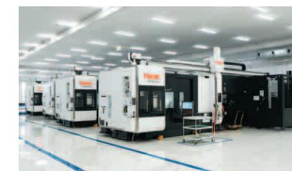
FMS line of the INTEGREX i series installed in Sankyo Dream Factory
