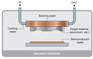
\* Target materials: Materials used for the film deposition of semiconductors
