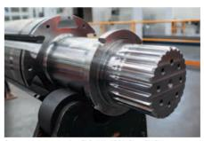
Spline and slotting detail on FLSmidth ABON Sizer Shaft
