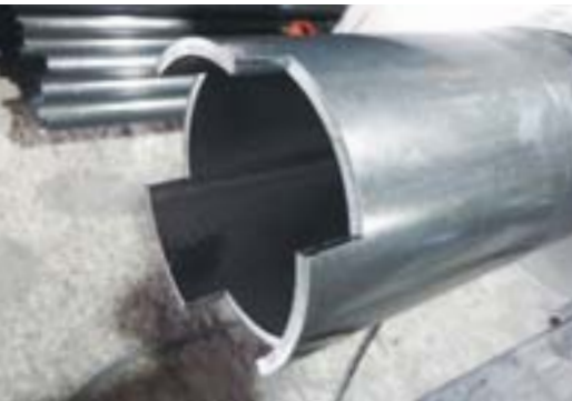
Steel pipe cut by 3D FABRI GEAR 220 II
