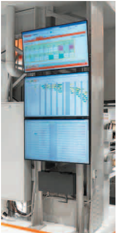
Large screens installed in the assembly area display the progress of processes on a real-time basis
