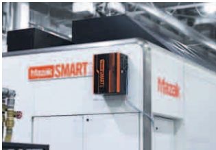
All data of machines are collected using the MAZAK SMARTBOX™ deployed in different locations of the machining area
