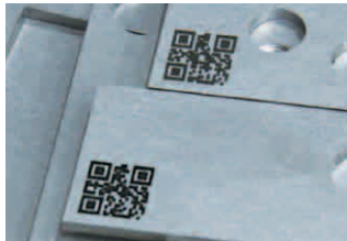
QR codes* are scribed by a laser processing machine *QR code is a registered trademark of DENSO WAVE INCORPORATED
