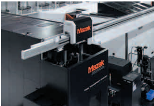
Tools are automatically supplied to multiple machines
