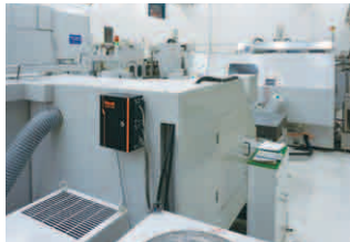
Information for older machines is collected by the MAZAK SENSOR BOX
