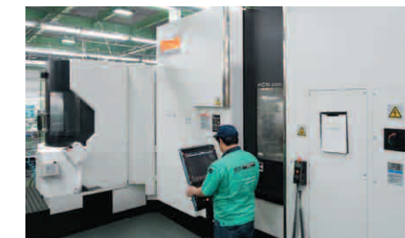
Mazak's horizontal machining center HCN-6000 with a 6-pallet changer performs unmanned operation over extended periods of time
