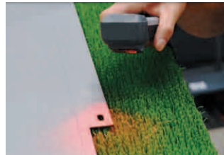
The operator calls the bending processing program by scanning the QR codes scribed on workpieces
