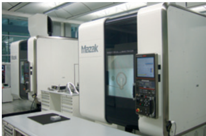
Two HYPER VARIAXIS 630 utilized for the machining of race car components
