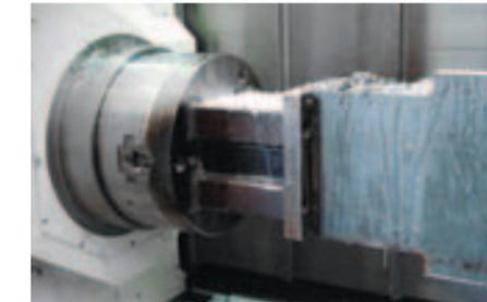
Fixture made by Austbore attached to machine chuck, further increases work efficiency and machining precision
