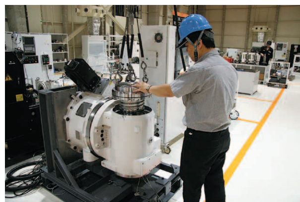
Milling spindle cartridge on test stand
