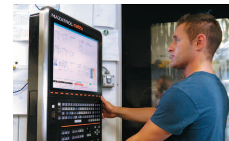
Operator programming a MAZATROL CNC
