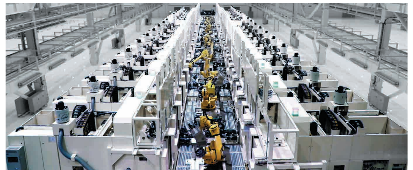
Mass production line for machining parts of automotive engines, which is composed of the FF-5000/40 horizontal machining centers and articulated robots
