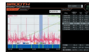
显示每台机床功耗的 Smooth Energy Dashboard
