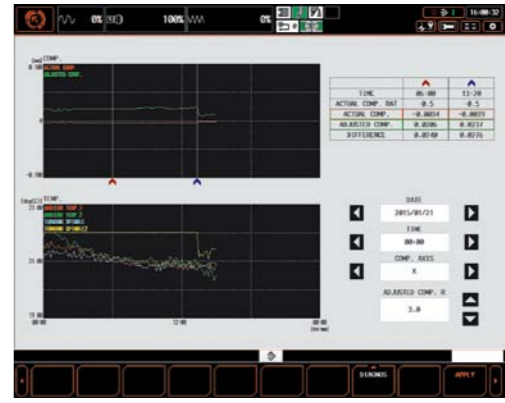
Temperature and compensation is displayed on screen. Operator can adjust compensation by looking at the data.
